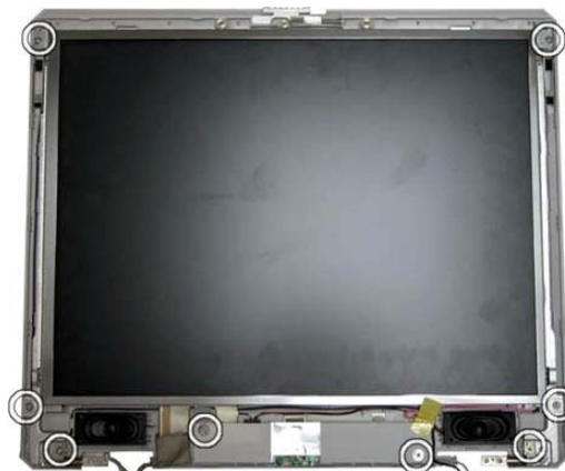
Fig. 24 Removing LCD panel and inverter board screws
